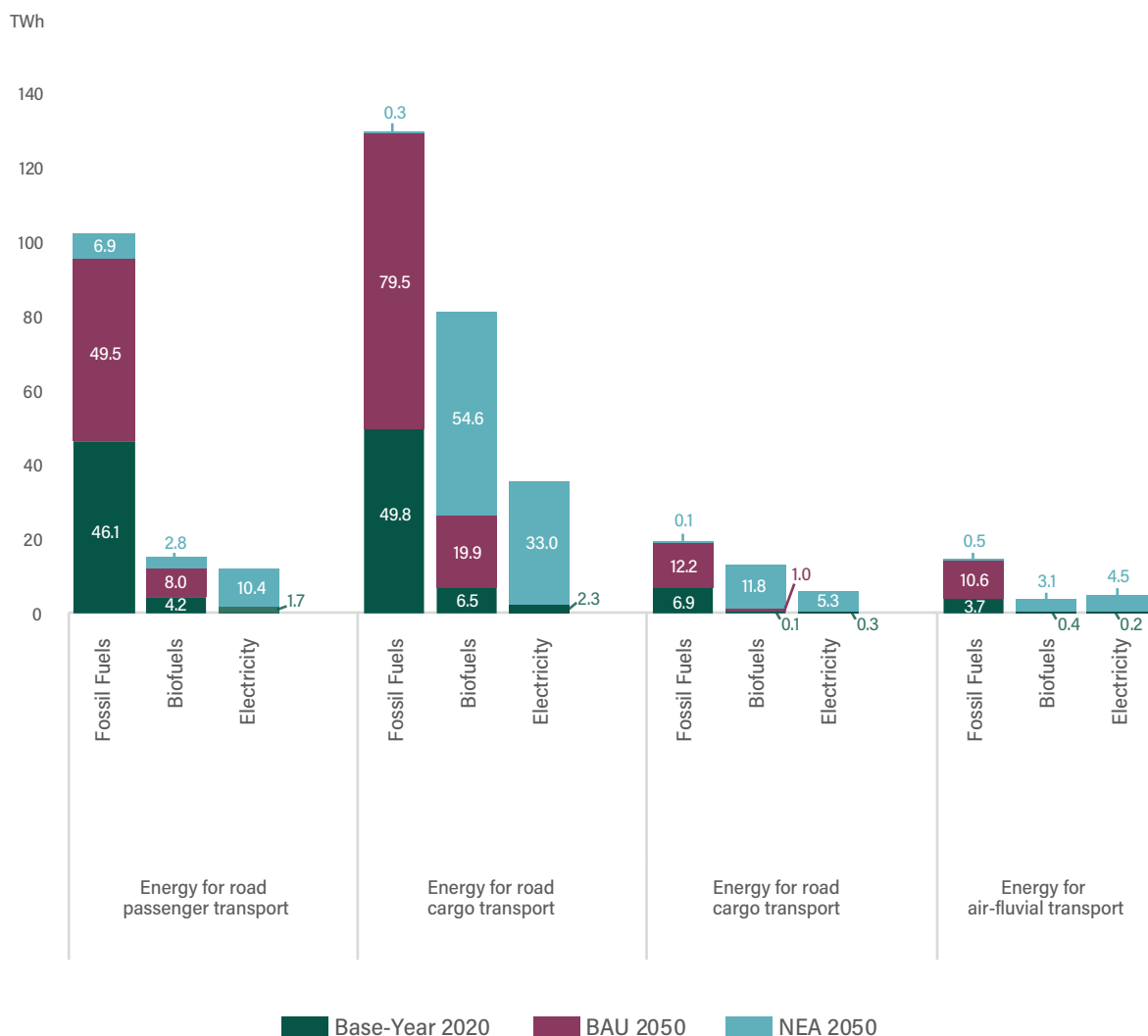
Chart 12 | Energy demand (TWh) by type of fuel, for each transport modality, simulated for the different scenarios and base year 2020
